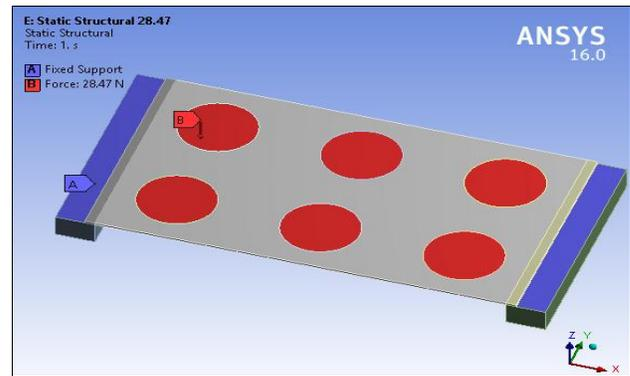
Fig. 6 Boundary Conditions for Simply Supported Crisper Plate
