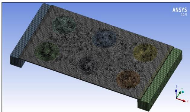
Fig. 5 Mesh Model (Simply Supported Crisper Plate)
