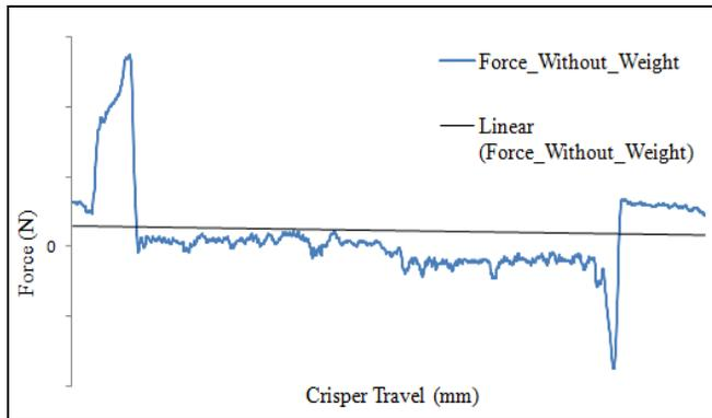
Fig. 18 Pull/Push Force Required (Without Load)
