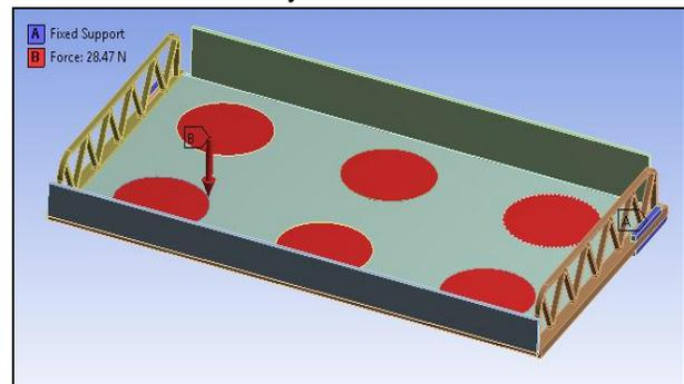
Fig. 10 Boundary Conditions for Modified Cantilever Crisper Plate
