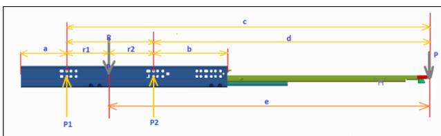
Fig. 3 Load Conditions and Reaction Forces on Glide
