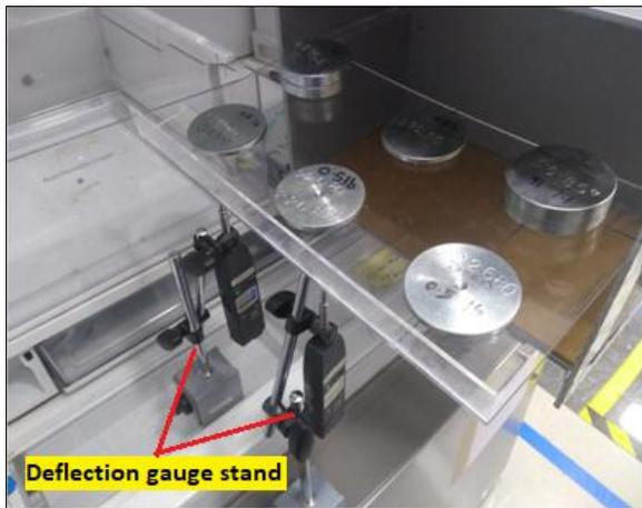
Fig. 15 Cantilever Condition Test Setup
