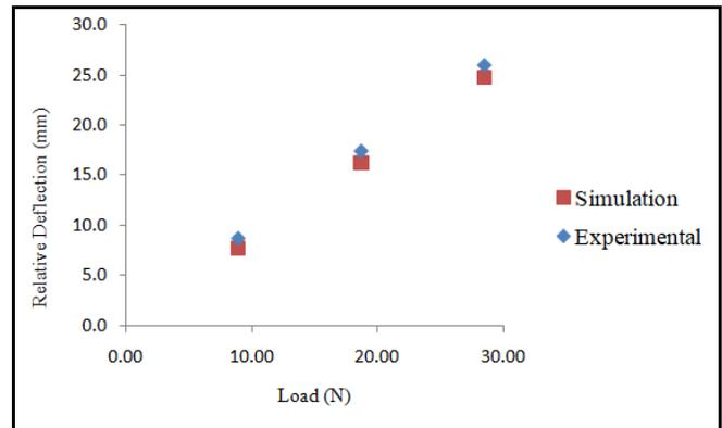
Fig. 20 Relative Deflection Vs Load Graph for Cantilever Condition of Plate
