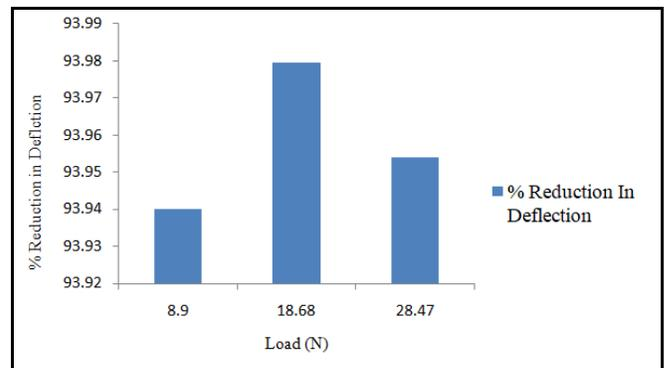
Fig. 21 Comparison of Deflection for Modified and Old Crisper Plate
