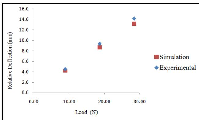
Fig. 19 Relative Deflection Vs Load Graph for Simply Supported Condition of Plate
