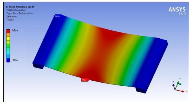
Fig. 7 Static Structural Analysis: Deflection Contour Plot for Simply Supported Crisper Plate
