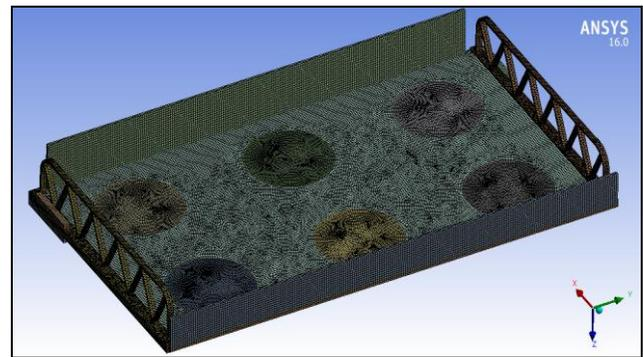
Fig. 9 Mesh Model of Modified Crisper Plate
