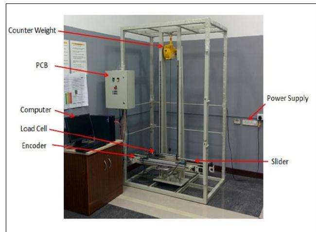
Fig. 16 Sensorial Fixture for Pull/Push Force
