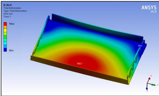
Fig. 11 Deflection Contour Plot for Cantilever Crisper Plate.
