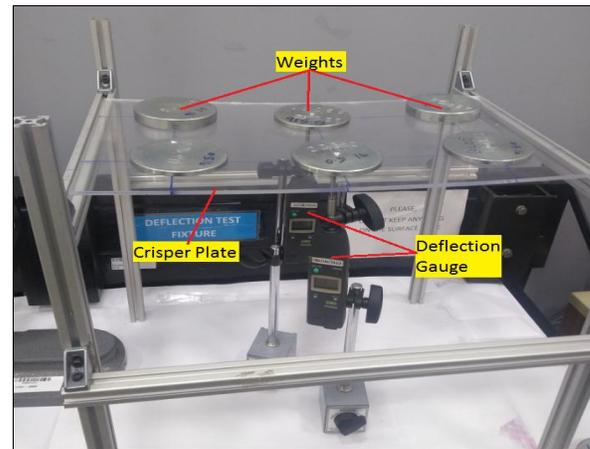
Fig. 14 Simply Supported Condition Test Setup
