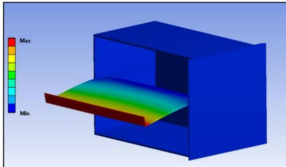
Fig. 8 Static Structural Analysis: Deflection Contour Plot for Cantilever Crisper Plate.
