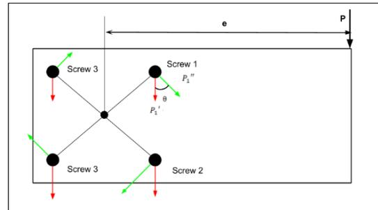
Fig. 4 FBD of Forces Acting on the Screw
