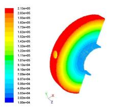
Fig. 11. Velocity vector colored by dynamic pressure (Pa)
