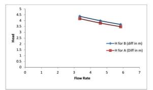
Fig.-15 Graph between flow Vs Head at 2600 rpm
