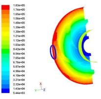
Fig. 5 Total pressure on blades profile (Pa)
