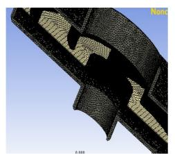
Fig 2: Sliced view of Impeller and casing (type A), Computational grid of Impeller (type A)
