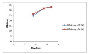
Fig.-22 Graph between flow Vs Efficiency at 2925 rpm
