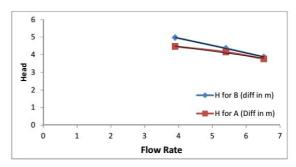
Fig.-17 Graph between flow Vs Head at 2825 rpm
