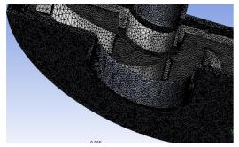
Fig 9: Sliced view of Impeller and casing (Type B) Computational grid of Impeller (type B)
