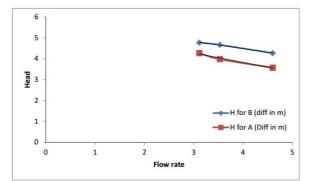
Fig.-16 Graph between flow Vs Head at 2700 rpm
