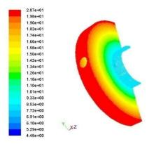
Fig.- 10. Velocity vectors colored by velocity magnitude (m/s) with casing
