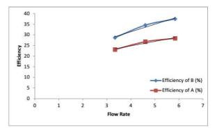
Fig.-19 Graph between flow Vs Efficiency at 2600 rpm
