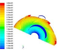
Fig. 7 Velocity vectors colored by velocity magnitude (m/s) on impellers blades, without casing
