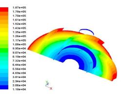
Fig.-6 contours of dynamic pressure (Pa)
