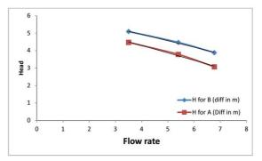
Fig.-18 Graph between flow Vs Head at 2925 rpm
