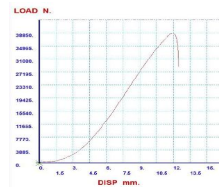
Figure 12. Graph load vs displacement 10 ply specimen
