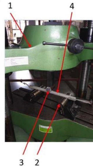
Fig. 4: Anti-intrusion beams testing equipment; 1 – Universal testing machine; 2 - cylindrical support; 3 - punch; 4 - anti-intrusion beam
