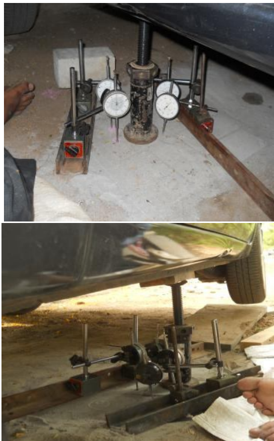
Figure 7. Deflection Measurement in Basket Weave and honey style Pattern
