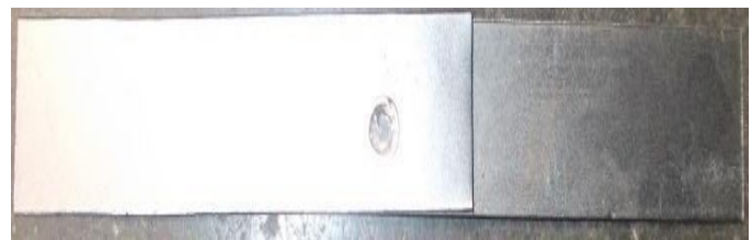
Figure 6. Work piece after finished spot welding
