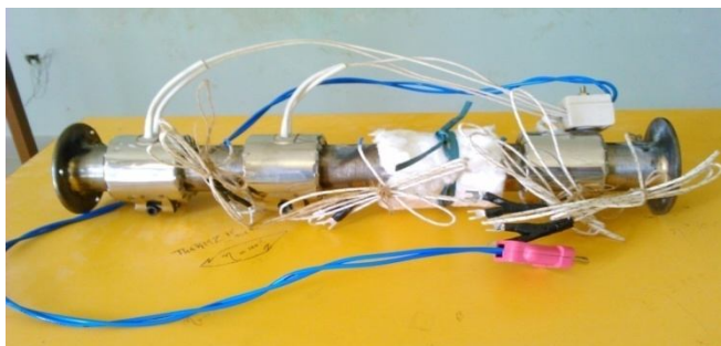
Fig.2.4 Test specimen having three band heaters
