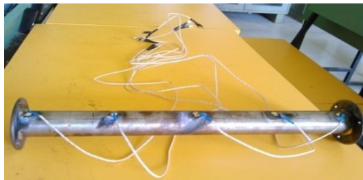
Fig 2.3 Test section with thermocouple
