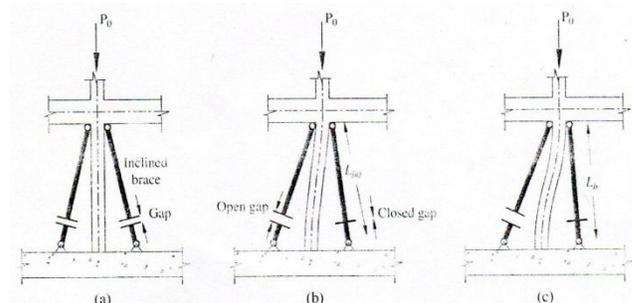
Fig.1 Mechanisms of Gap Inclined Brace
