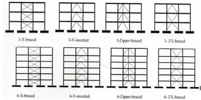
Fig.2 Bracing Models
