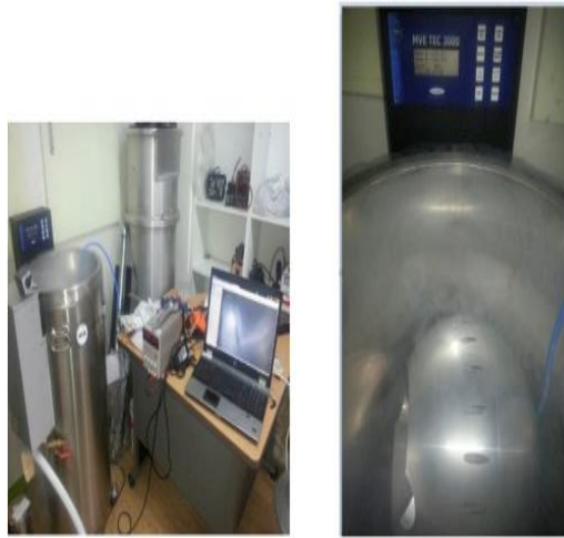
(a) Experiment equipment (b) Cryogenic camera in LN 2 tank Fig. 10. Test of cryogenic camera in LN 2 tank.
