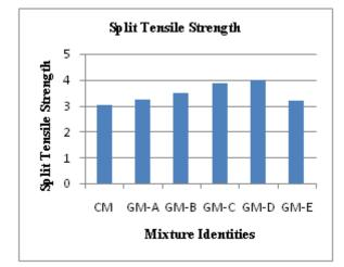
Figure.2 Graphical Representation of Split Tensile Strength of Cylinder
