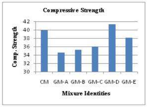
Figure.1 Graphical Representation of Compressive Strength of Cube
