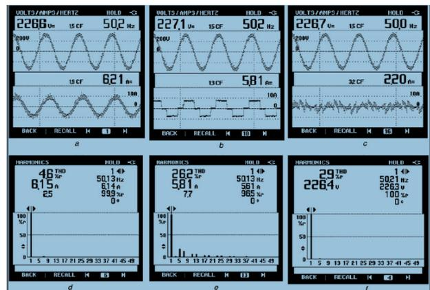
Fig. 6 Performance of the DSTATCOM under non-linear loads
