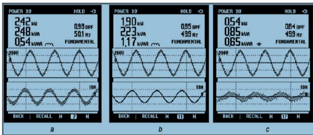
Fig. 3 Performance of the DSTATCOM under linear loads
