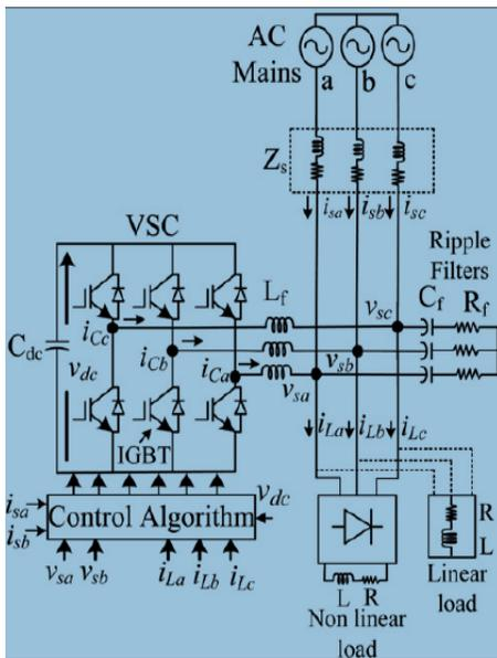
Fig. 1 Schematic diagram of the VSC-based DSTATCOM
