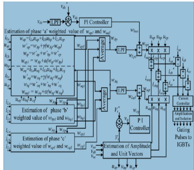
Fig. 2 LVQ control algorithm for DSTATCOM
