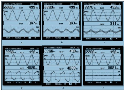
Fig. 7 Performance of the DSTATCOM under unbalanced non-linear loads
