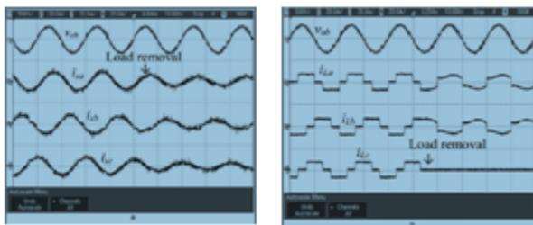
Fig. 8 Dynamic performance of the DSTATCOM during removal of phase 'c' in non-linear loads
