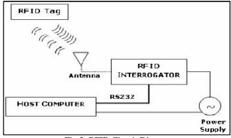
Fig.2. RFID Circuit Diagram
