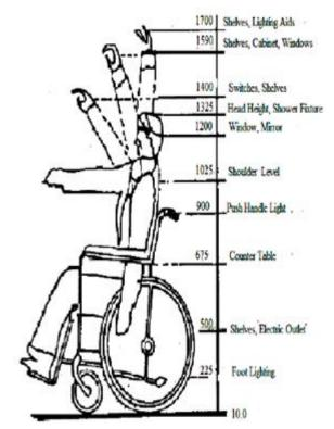
Fig. 1: Basic Wheelchair and its arm reach (A Review on Development of Wheelchair cum Stretcher)
