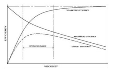
Graph 1: Efficiency v/s Viscosity (Hydraulic Fluid Properties and its influence on system performance)
