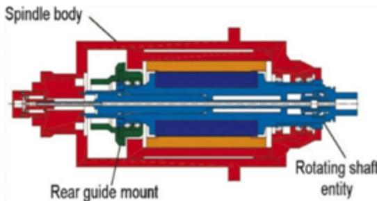
Fig. 4. The HSM spindle bearing system.
