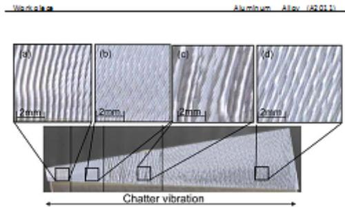
Fig.1. Machined surface after milling test.
