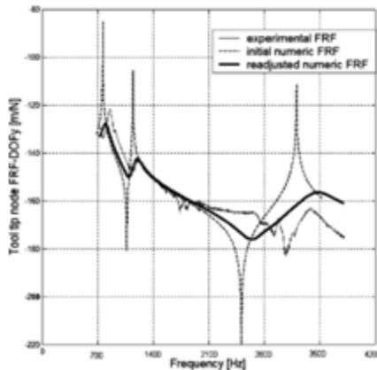
Fig. . Experimental, initial and readjusted FRF.
