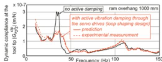
Fig 3: Tool compliance without and with active vibration damping (a)
