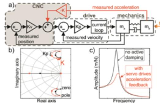
Fig. 2. Vibration damping by velocity set point acceleration feedback: Control diagram, (b) velocity loop root locus and (c) tool tip compliance
