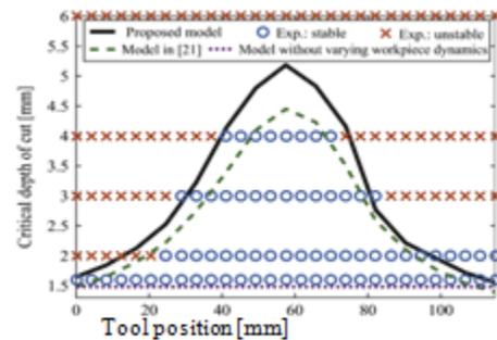
Fig. 6. Comparisons of stability borders obtained by different models.
