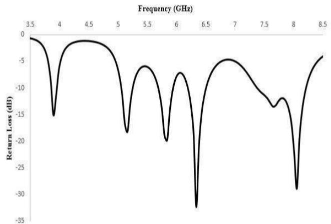
Fig-2 Return Loss of Patch 1
