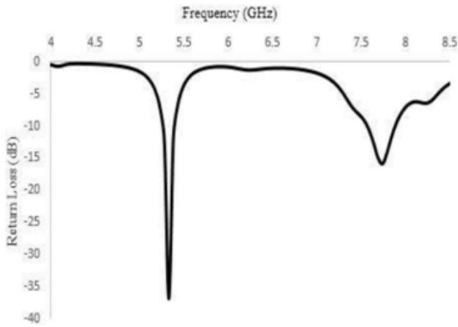
Fig-3 Return Loss of Patch
