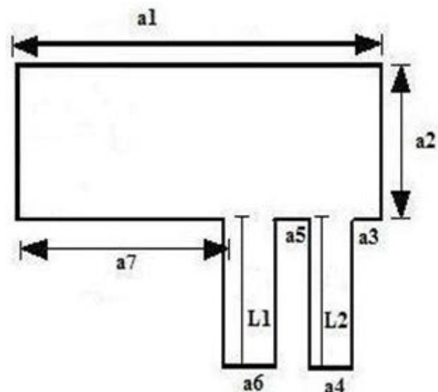
Fig -1 Geometry of the proposed rectangular patch antenna
