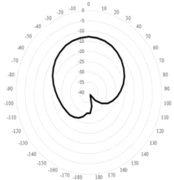
Fig-6 Radiation Pattern at 4.8 GHz
