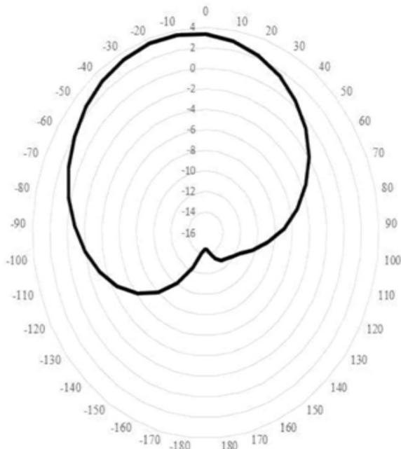
Fig-5 Radiation Pattern at 2.4 GHz
