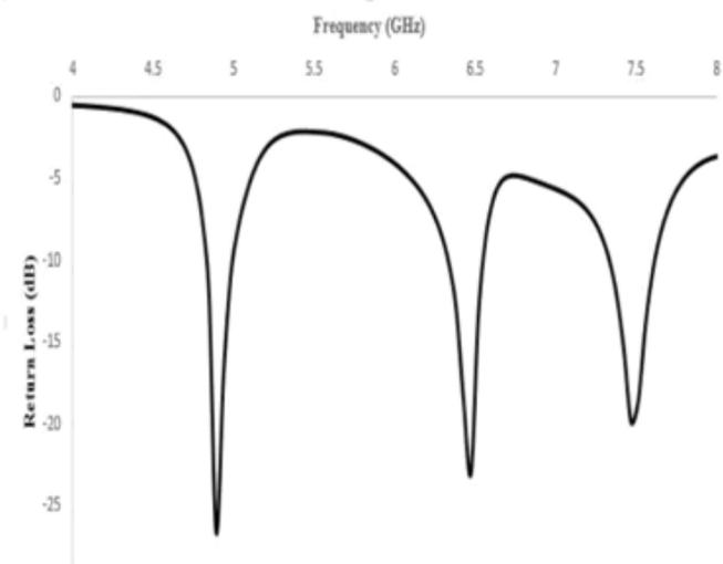
Fig-4 Return Loss of Patch 4
