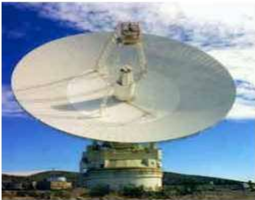
Fig 2. Parabolic reflector antenna
