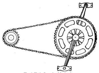
Fig. 1 Chain Sprocket Mechanism
